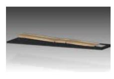
Made of treated Douglas fir or Heart of Douglas fir. 5.00 m modular panels, made of non-slip grooved planks 145 x 36 mm, mounted on joists. Passage width 1.50 m Space for the wheels: 80 x 80 mm
