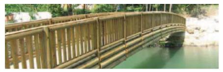
Curved mixed wood & steel gangway. Curved galvanized steel structure, dimensions according to Eurocode 3, wooden cladded. Grooved wooden decking, 36 mm thick.
