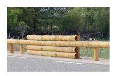
Built from our T22 2M or T22 4MS2 mixed wood & steel guardrail, 4-height railing with C125 post on a steel base. Height 1 m above ground.
