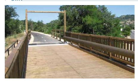
Straight mixed wood & steel gangway. Galvanized steel structure, dimensions according to Eurocode 3, wooden cladding. Grooved wooden decking, 50 or 80 mm thick. Mixed Wood & Steel Parapets T100 or T140, tested according to the norm XP
