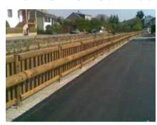
Tested according to French standard NF P01-013, NF P01-012, meeting norm XP P98-405 safety requirements. Galvanized steel post on steel base with wooden cladding: 2 m post spacing. Wooden panel with barrels. Panel connected to barrels and post with galvanized steel parts 1.03 m above ground Combined with mixed wood and steel guardrail T18 or T22. Adjustable for cutting and curves and level differences
